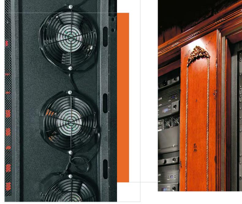
thermal management Thermal Management plays a critical role in overall system reliability because heat has been proven to substantially reduce the service life of most equipment. Maintaining the recommended constant operating temperature for most equipment (max 85°) will help provide a long service life for the equipment inside an enclosure. Why 85°? Most studies have shown that for every 10° rise, digital equipment life is reduced by approximately 40%!
